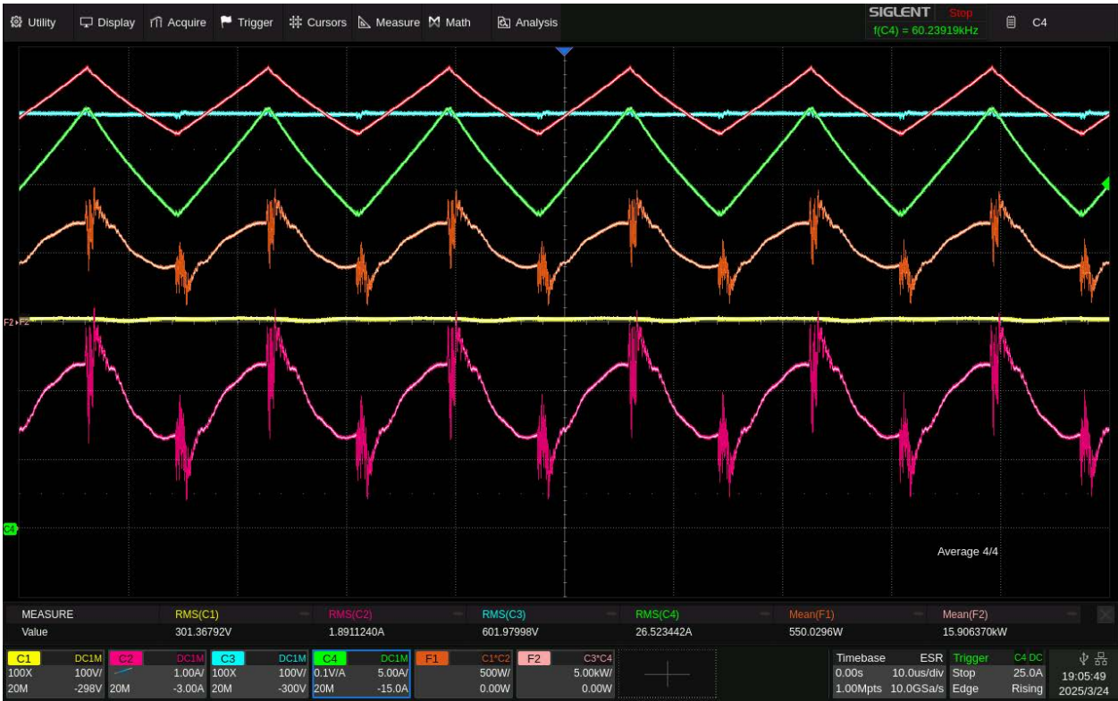
Figure 21: Oscilloscope Overview for Output of 600V and 25A with Switching Frequency of 60 kHz
