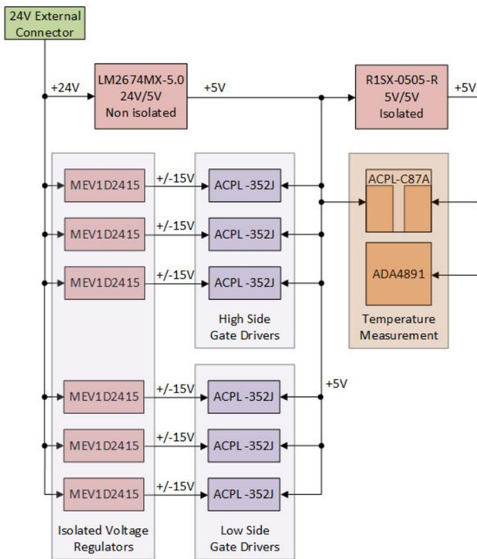
Figure 5: (a) 24V/5V Power Supply of the EB1200-352J Board, and (b) the Isolated 5V/5V Power Supply
