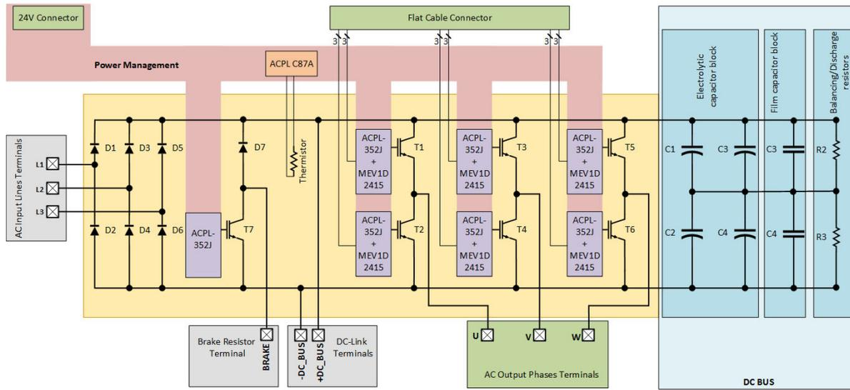
Figure 3: Functional Block Disposition of the EB1200-352J
