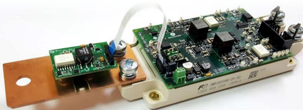
Figure 1: Evaluation Gate Driver Board EB1200-339J and ACPL-736J Sigma Delta Current Sensing Module
