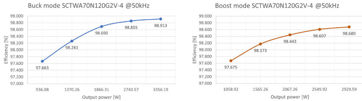
Figure 23: Measured Efficiencies of Buck (Left) and Boost (Right) Mode Operation with STM SCTWA70N120G2V-4 SiC MOSFET Devices at 50-kHz Switching Frequency
