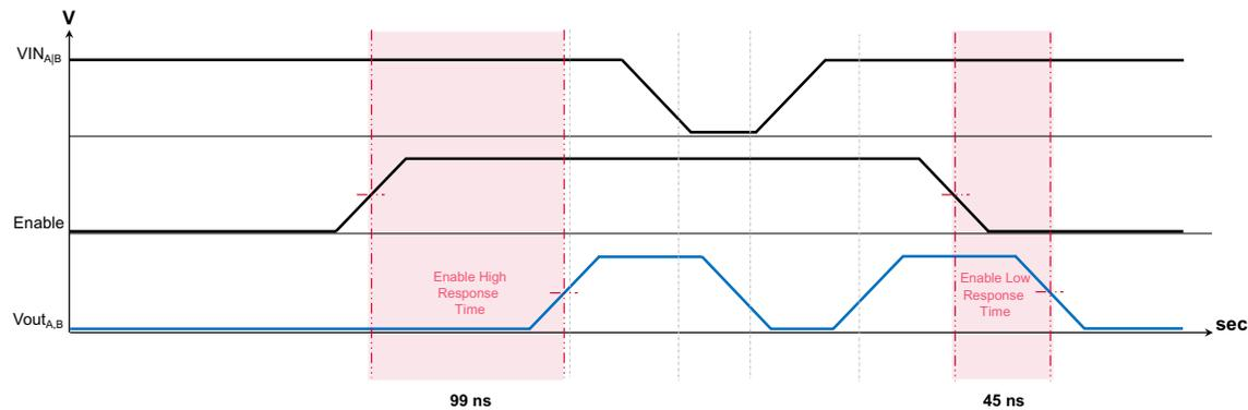
Figure 35 shows the response time that the enable function has on the dual-channel outputs. The enable function adds on a 50-ns delay on the rising edge of the output, but not on the falling edge.
