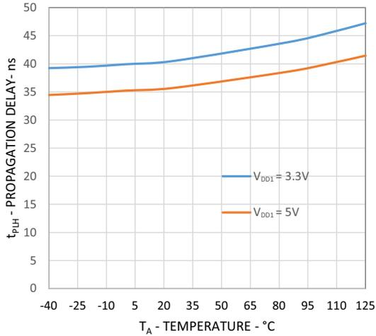
Figure 13:  $t_{pHL}$  vs Temperature
