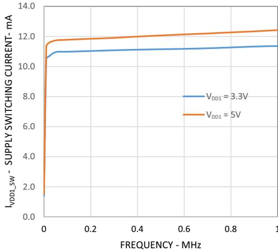
Figure 27:  $I_{VDDA,B}$  vs  $V_{IN_A}$  &  $V_{IN_B}$  Input Switching Frequency
