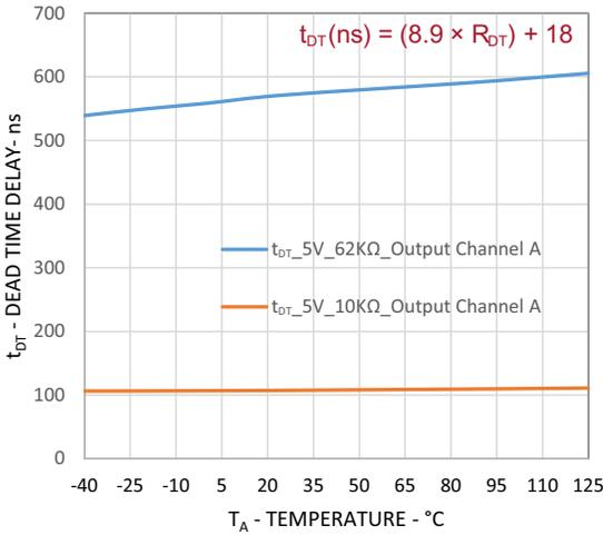
Figure 31: Dead Time Matching vs. Temperature
