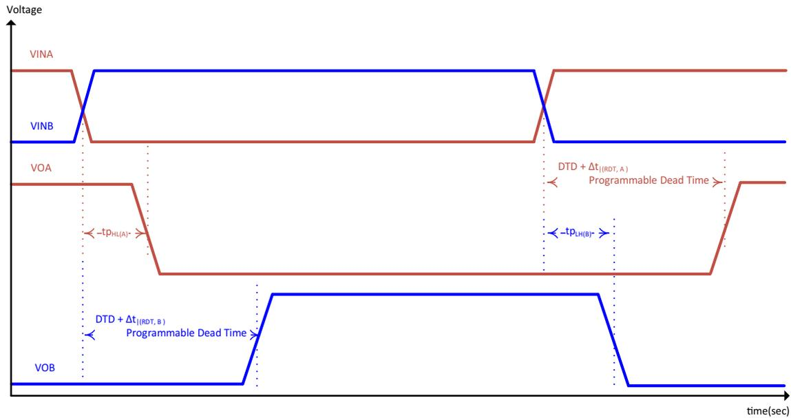
Programmable dead time is set according to the equation  $t_{DT}$  in (ns) =  $(8.9 \times R_{DT}) + 18$ ,  $R_{DT}$  in  $k\Omega$ . The measured dead time at both the gate driver outputs  $V_{OA}$  and  $V_{OB}$  are the total of the programmable dead time plus the dead time distortion (DTD).
