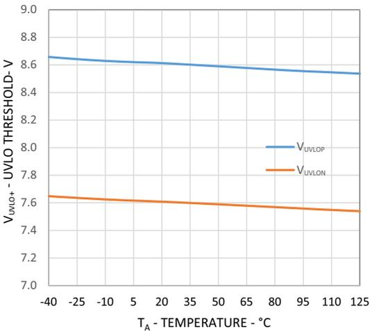
Figure 17:  $UVLO_{A,B}$  Hysteresis vs Temperature
