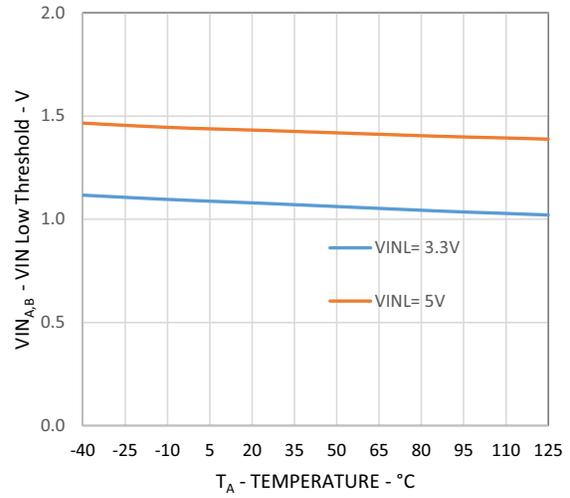
**Figure 20: VIN Hysteresis vs Temperature**
