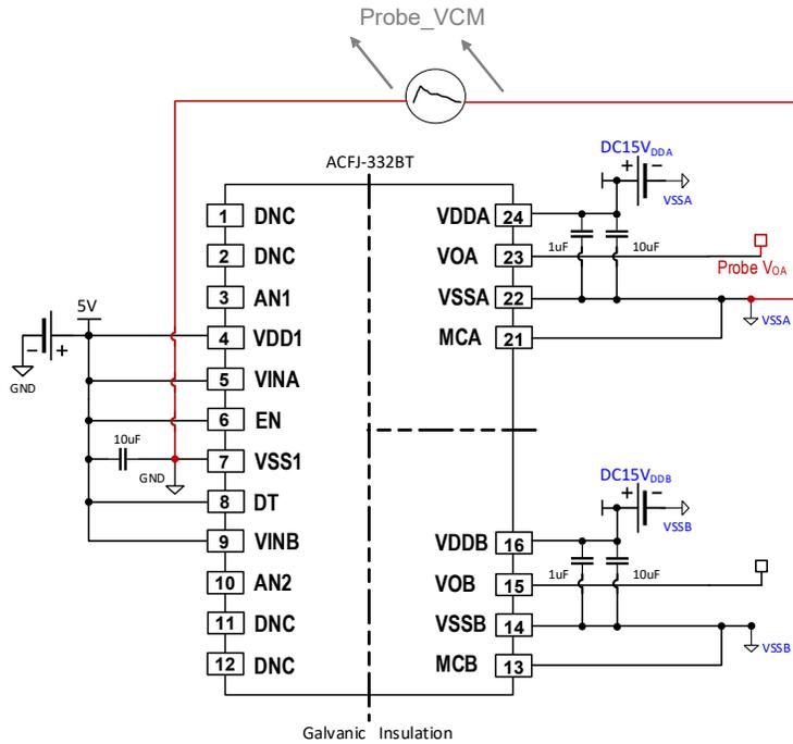
Figure 8: CMR  $V_O$  Low Test Circuit
