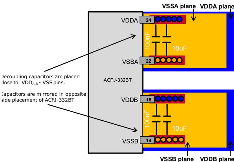
Decoupling capacitors are placed close to VDD<sub>A,B</sub> - VSS pins.
