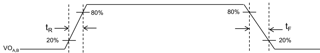
Figure 6: Rise and Fall Time Measurement
