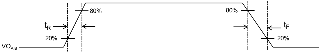
Figure 6: Rise and Fall Time Measurement
