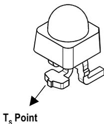
$T_S$  can be easily measured by mounting a thermocouple on the soldering joint as shown in [Figure 15](#), while  $R_{\theta J-S}$  is provided in the data sheet. Verify the  $T_S$  of the LED in the final product to ensure that the LEDs are operating within all maximum ratings stated in the data sheet.
