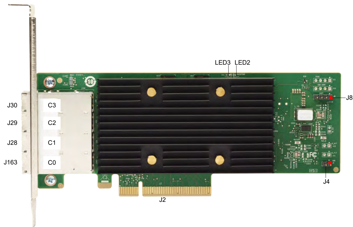
Figure 15: Card Layout of the eHBA 9600-16e Storage Adapter
