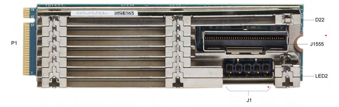
Figure 10: Card Layout for the MegaRAID 9524-8i Tri-Mode Storage Adapter
