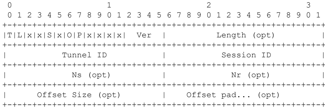
Figure 42: L2TPV2 Header
