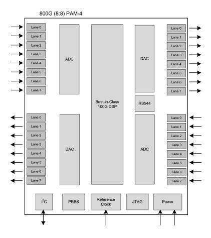
Figure 2: Application Diagram
