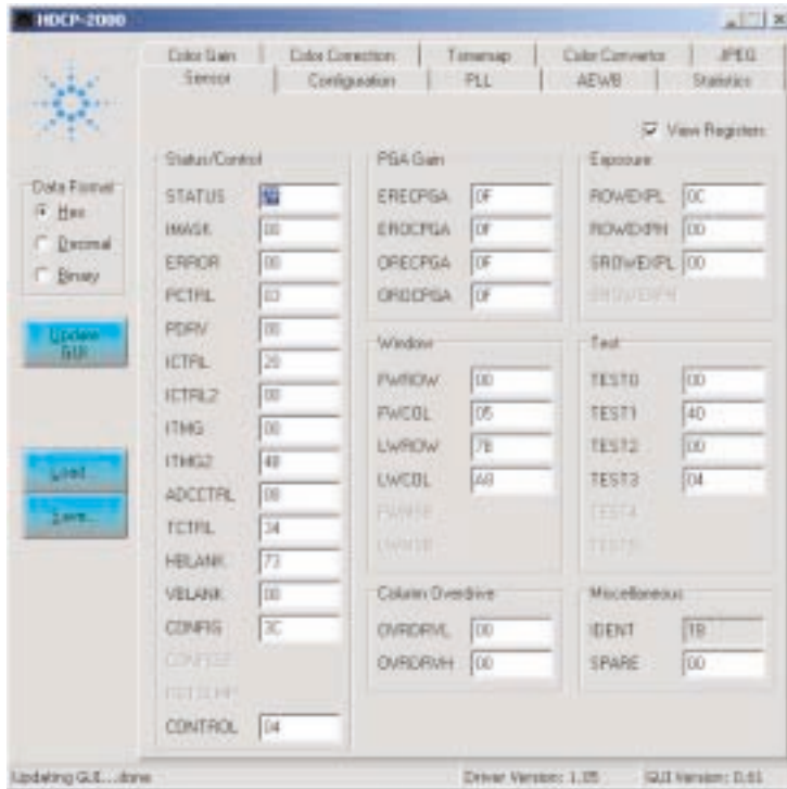
Figure 7. Sensor register setting screen.
