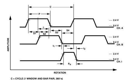
S1... S4 = LOGIC STATE WIDTH (4 STATES PER WINDOW AND BAR PAIR, EACH STATE IS 90°e)
