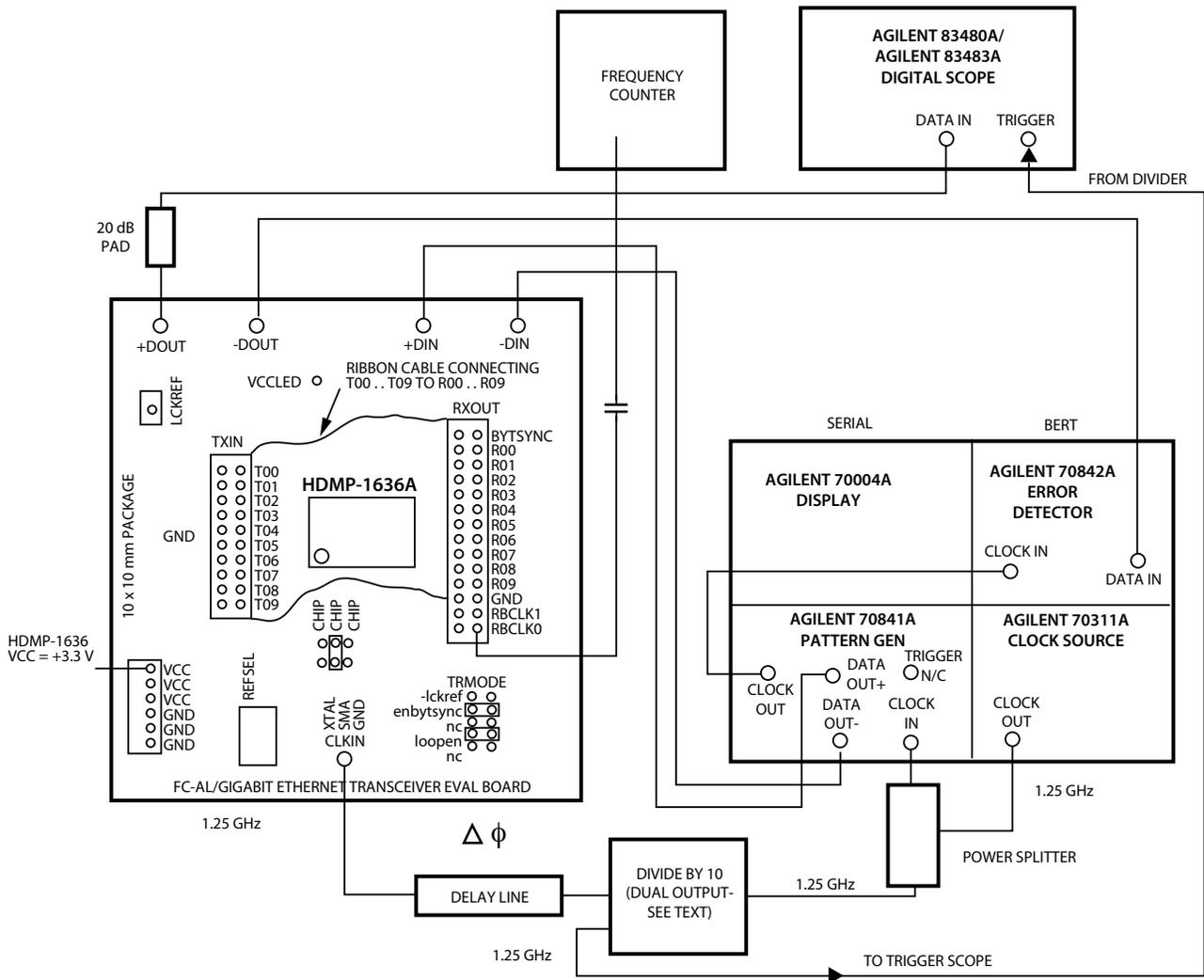
Figure 3. BER Test Setup using the HDMP-1636A Evaluation Board and Avago Technologies' Serial BERT.
