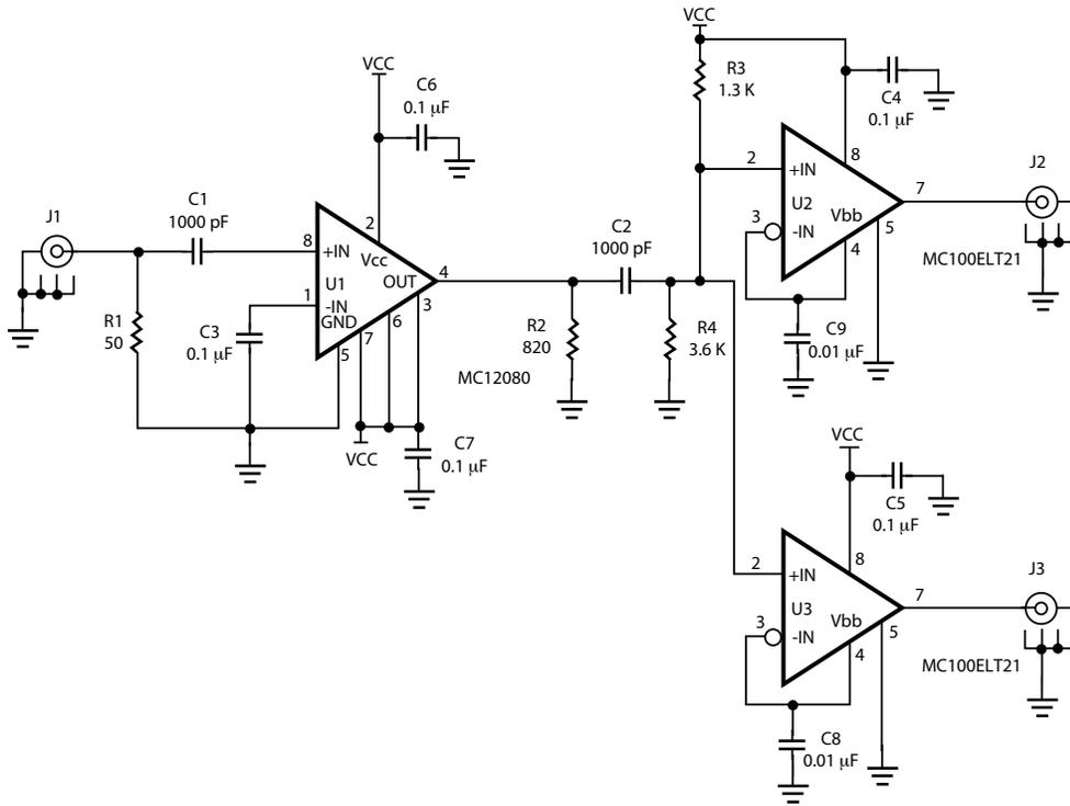
Figure 5. Divide by 10 Network used with the BER Test.
