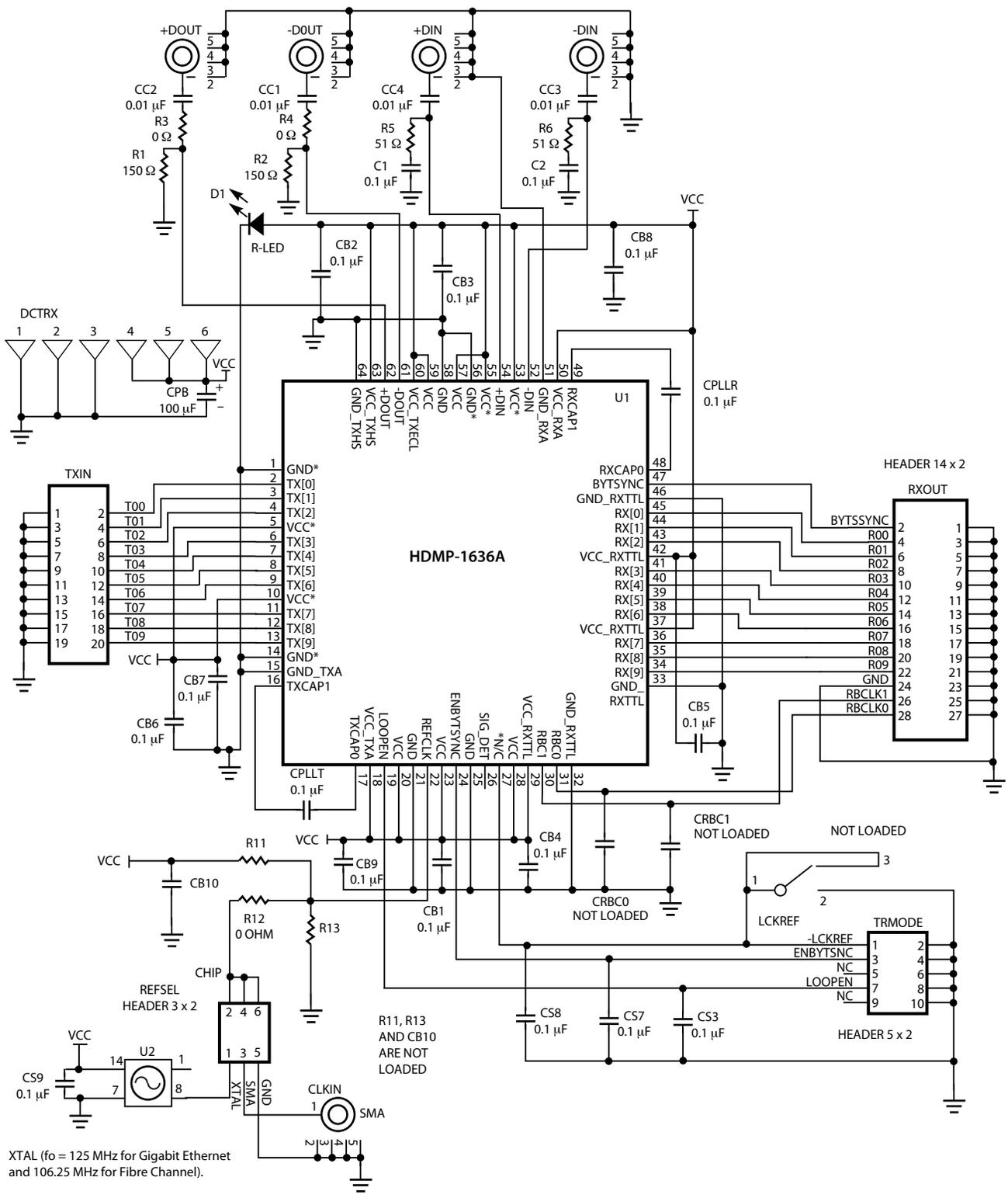
XTAL (fo = 125 MHz for Gigabit Ethernet and 106.25 MHz for Fibre Channel).
