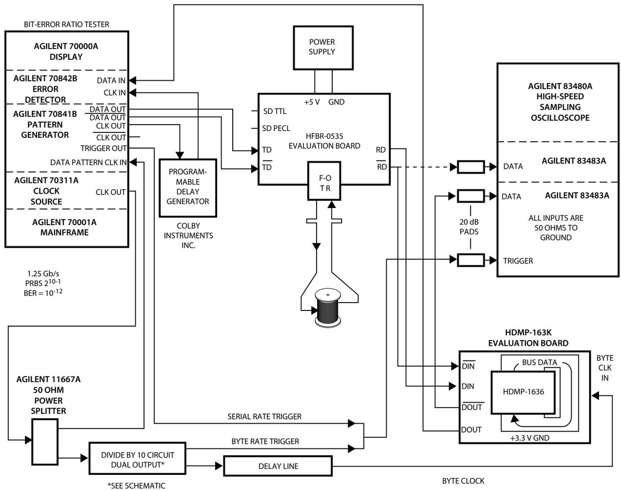
Figure 6. Recommended Test Configuration for One Looped-back HFBR-53D5 or HFCT-53D5 Fiber-optic Transceiver Link with a Looped-back Parallel Bus Gigabit/sec Ethernet HDMP-1636A Transceiver IC.
