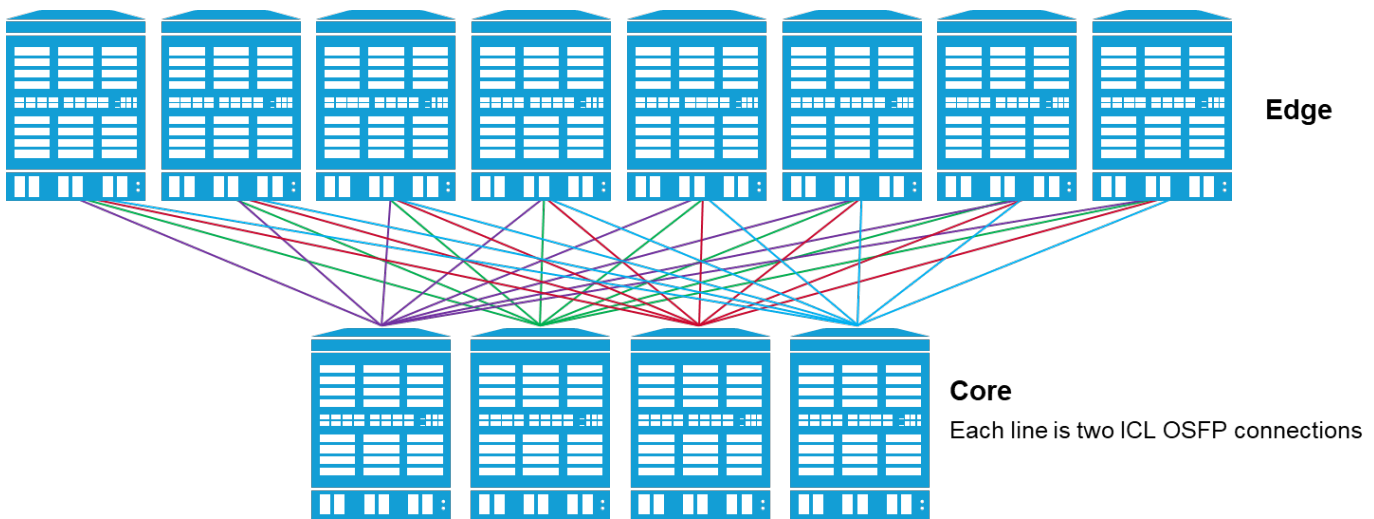
Figure 5: UltraScale X8-8 ICL Core-Edge Architecture
