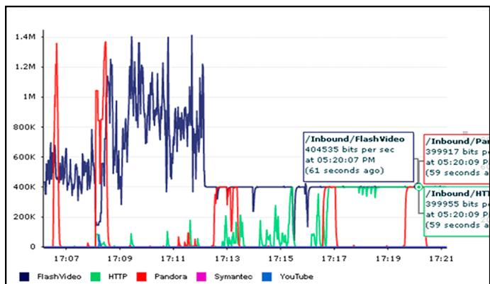
In this graph we see a spike in YouTube traffic that consumes most of a T-1 link, disrupting other applications. A shaping policy is implemented, capping the traffic and restoring performance for key applications.
