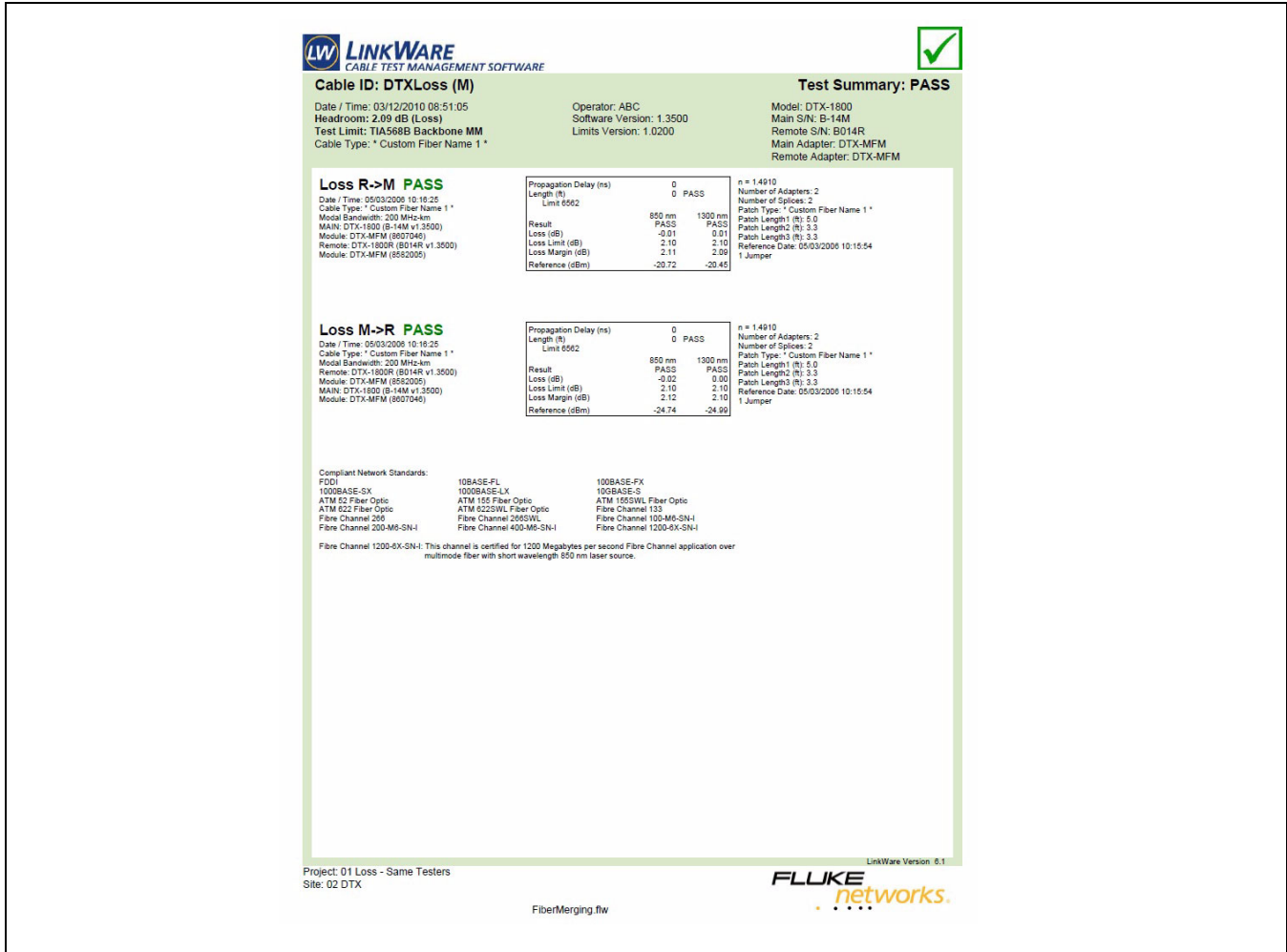
Figure 9: Fiber Certification Test Result Example
