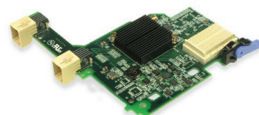
IBM 10GbE VFA II for IBM BladeCenter HS23 Provided by Emulex (IBM PN 81Y3120)
