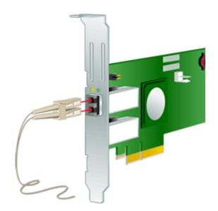
Figure 3: Connecting Fiber Optic Cable
