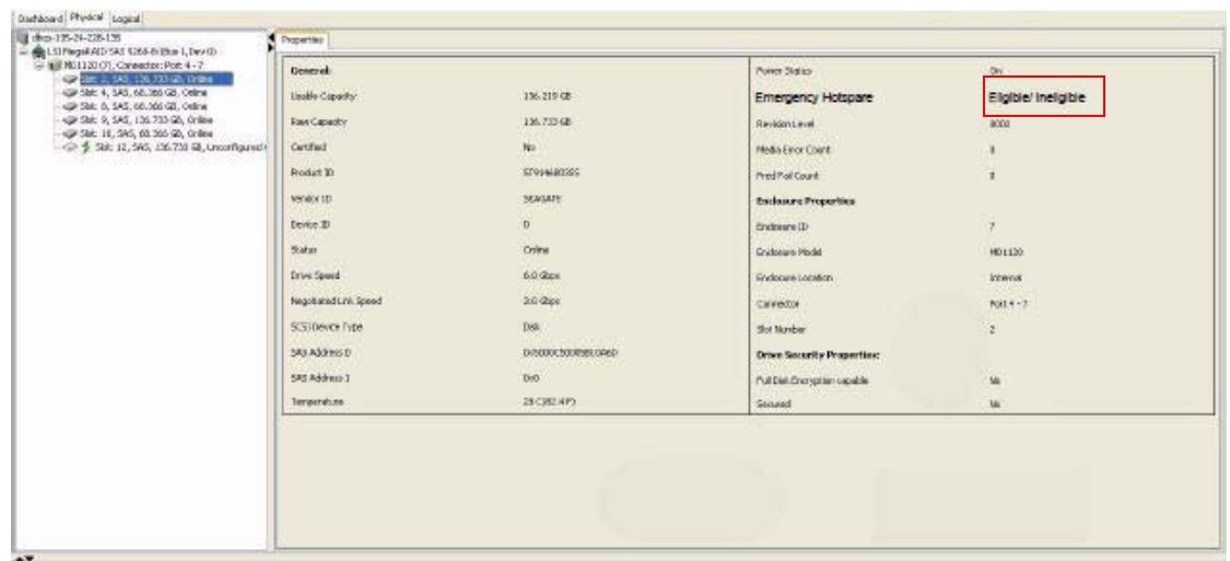
Figure 187: Emergency Hot Spare – Physical Drive Properties
