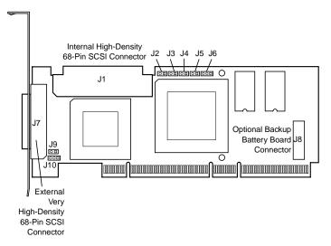
Step 4: Install the MegaRAID SCSI 320-1 Controller
