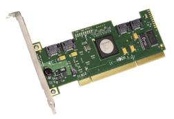
Thank you for purchasing the LSI Logic SAS3041X-R Serial Attached SCSI (SAS) to PCI-X Host Bus Adapter (HBA). Please take a few minutes to read this *Quick Installation Guide* before you install the SAS3041X-R.
