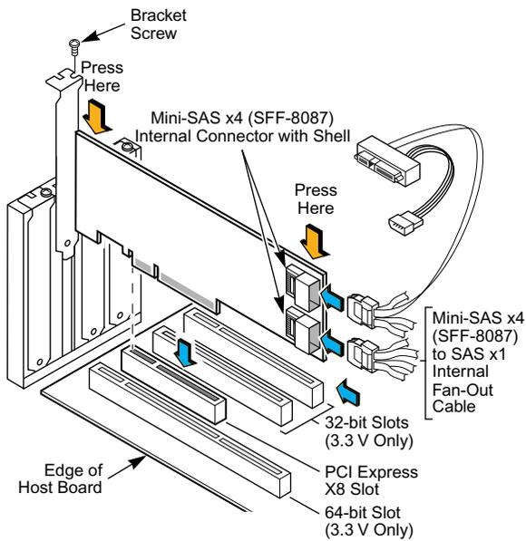
**NOTE:** The shape, size, and locations of the components on your HBA and its bracket might vary from this illustration. The HBA requires a x8 PCIe slot.
