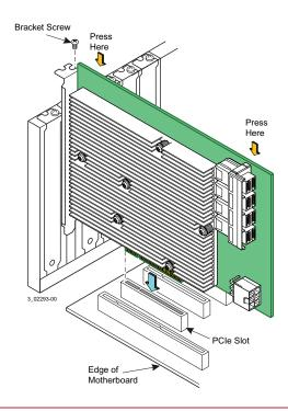
NOTE: The shape, size, and locations of the components on your HBA and its bracket might vary from this illustration. The HBA requires a x8 PCIe slot.
