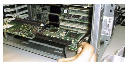
Figure 2-8. Plug the Controller into any 32-bit or 64-bit PCI Slot
