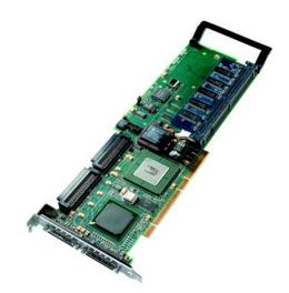
Figure 1-1. AcceleRAID 352 Controller
