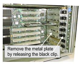
Figure 2-6. Remove the Metal Plate
