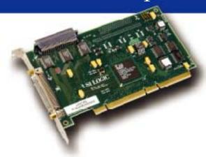
The LSIU160 Ultra160 SCSI host adapter is the best solution to connect to high performance Ultra160 hard disks drives.
