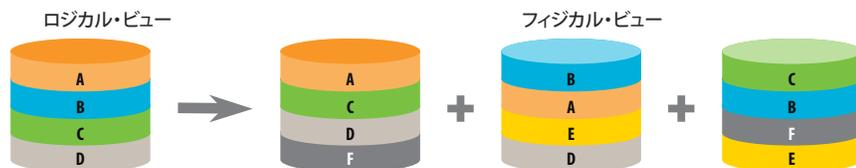
図3. Integrated Striping (RAID 0)
