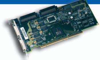
The LSI22915A Ultra160 SCSI host adapter offers the highest Ultra160 SCSI performance with two internal and external channels.
