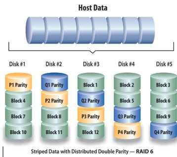
**RAID 6:** Two sets of parity data, P + Q, are striped across disks. RAID 6 safeguards against data loss during rebuild mode by allowing up to two consecutive drive failures for maximum fault tolerance.
