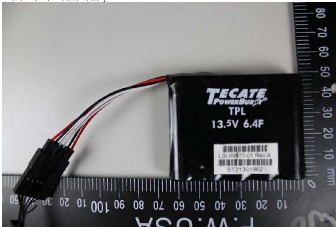
Front View of Tecate Battery
