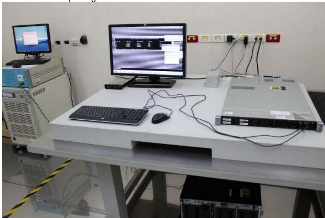
View of Harmonics/Voltage Flicker Test
