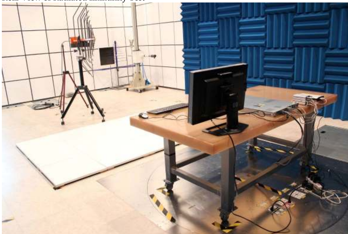
Rear View of Radiated Immunity Test
