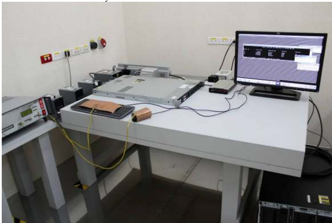
View of Conducted Immunity Test
