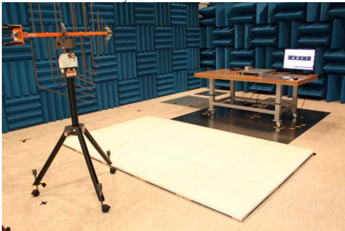
Front View of Radiated Immunity Test
