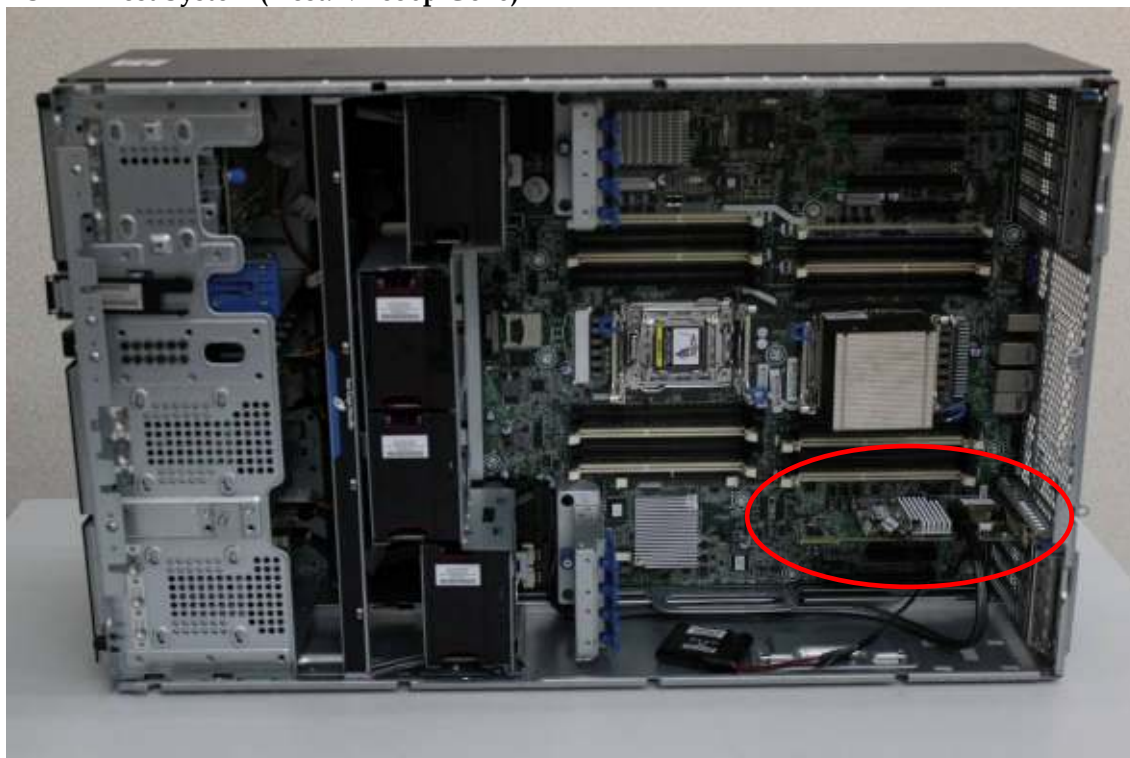
EUT in Host System (Host: ML350p Gen8)
