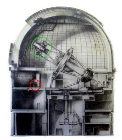
The 4 meter Blanco telescope. The eventual home of the Dark Energy Camera, DECam, which is planned to generate 400 1GB images per day, all of which are expected to be processed and stored on storage components from LSI, including the MegaRAID SAS 9260-8i controller with BBU, the LSI LSISS9252 SATA Adapters for Expanders and CacheCade software. The green circle marks the location of the prime focus cage where DECam will be mounted. The red circle marks a person, included for scale.
