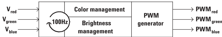
Figure 8. The ASSP samples the tricolor photo sensor directly and translates the readings into the required LED PWM signals.
